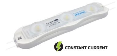
12VDC(Constant Voltage) driven ColibriLED module has a built-in microprocessor, that restricts the current to the nominal for each LED chip individually. This technical design expands the lifespan of ColibriLED module, protects LED chip from overpowering, equalizes the brightness of LED modules despite the position of the module in the chain.
